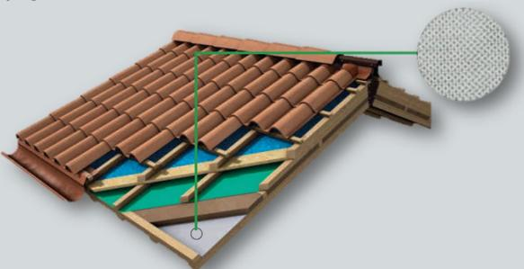
The surfaces to be protected must be dry, clean and sufficiently smooth or levelled, they must not have any protuberances that might puncture the underlay or compromise its adhesion to the substrate.
