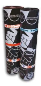
Monoreinforced waterproofing membrane made up of a compound based on distilled bitumen modified with plastomeric polymers reinforced with non woven polyester fabric. Reinforcement and special compounds ensuring high workability and good mechanical properties.
