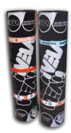
Monoreinforced waterproofing membrane made up of a compound based on distilled bitumen modified with plastomeric polymers reinforced with non woven polyester fabric. Special compound ensuring high flexibility at low temperatures mixed with special chemical components preventing plant root perforation.
