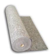
Geotextile fabric which is only made up of synthetic fibres connected to each other by means of a needle punching process without using any glue or chemical binder.
