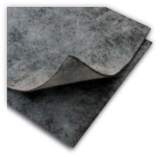
Vapour barrier made up of three layers of non woven fabric and polypropylene film specially designed to slow down the passage of air and water vapour through insulation layers, thus reducing the formation of condensation. It can be fully recycled providing high wind resistance.
