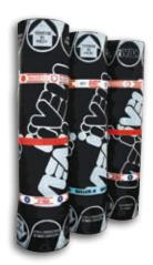
Monoreinforced waterproofing membrane made up of a compound based on distilled bitumen modified with plastomeric polymers reinforced with non woven polyester fabric.
