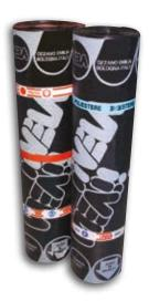
Monoreinforced waterproofing membrane made up of a compound of excellent quality based on distilled bitumen modified with high elasticity elastomeric polymers (BPE), reinforced with non woven polyester fabric.
