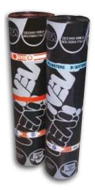
Monoreinforced waterproofing membrane made up of a compound based on distilled bitumen modified with plastomeric polymers reinforced with non woven polyester fabric. Reinforcement and special compounds ensuring high flexibility at low temperatures and good mechanical properties.
