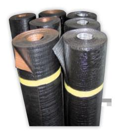
Glass fabric reinforced waterproofing membrane made up of a special compound based on distilled bitumen modified with elastomeric polymers (BPE), self-protected with copper or aluminium metal sheets with special embossing allowing free metal expansion. Surface finishing not only ensures good aesthetic appearance, but also reflects sunrays, thus protecting the membrane against atmospheric agents, highly reducing maintenance operations.
