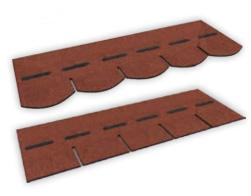
Bituminous shingles self-protected with ceramic-coated granules reinforced with fiberglass available in three profiles. The reinforcement provides good dimensional stability even in the presence of high temperature ranges. The upper surface of the shingles covered with ceramic-coated granules protects bitumen layers against UV rays and atmospheric agents.
